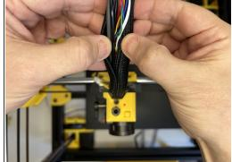
• Insert the 3mm nylon filament and tuck the cable harness in the cable sleeve.
