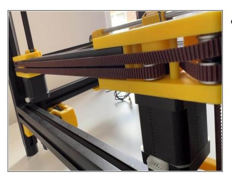
Check the belt positions on the back of the printer. They should be aligned with the idler pulleys.
