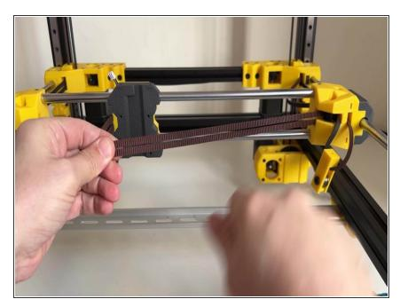
Hold the belts on the right side as you did with the left. Align the first part of the belt lock. Place the second part and tighten the M3 x 6mm locking screw.
