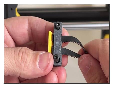
Use two M3 x 8mm screws to assemble the belt lock on the Extruder Carriage.
