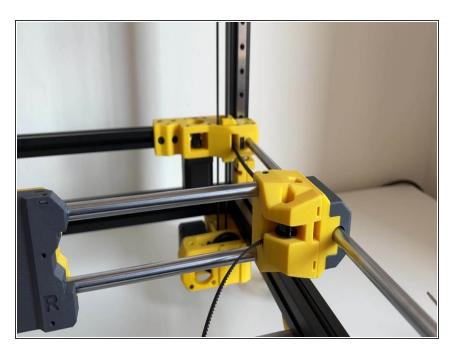
Start with passing the belt through XR Carriage and slip it in A Drive.
