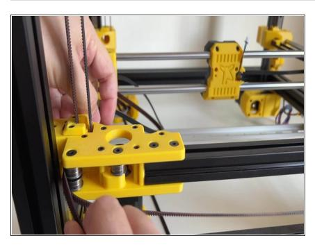
Pass the belt around A Drive Motor Pulley.
