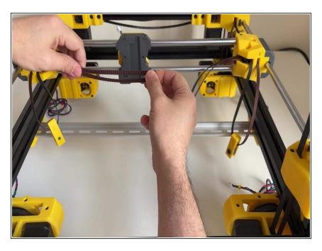
Get the belts and align the ends with the belt lock part. Leave a 5mm piece on both ends and hold it.
