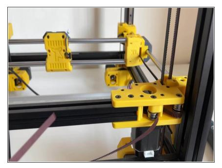
Pass the belt from B Drive and then XL Carriage. Bend the end tip of the belt slightly for a smooth pass through the idler pulley inside the XL. Belt will make a 90 degree turn towards the extruder.
