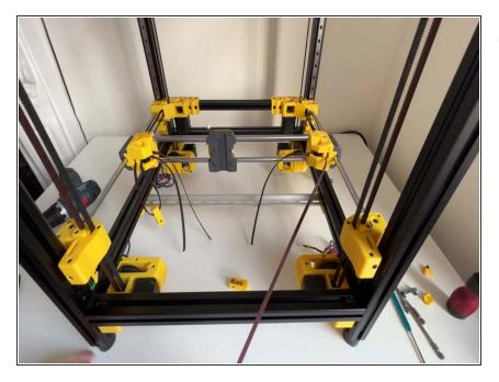
Pass the belt around the Right tensioner. As mentioned, both tensioners are identical. Just use the R side up when inserting into YR Carriage. Bend the tip of the belt slightly and slip the belt around the idler on XR. Try to align the belt with the pulley while pushing in.
