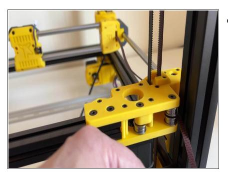
Pass the belt around the motor pulley.
