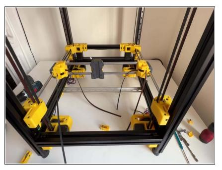
Pass the cable through the Left tensioner. Both tensioners are identical, you should use L side up when inserting to YL Carriage. And then pass the cable around the idler pulley but again bend the tip of the belt to ease the turn. Try to align the belt with the pulley when pushing in.
