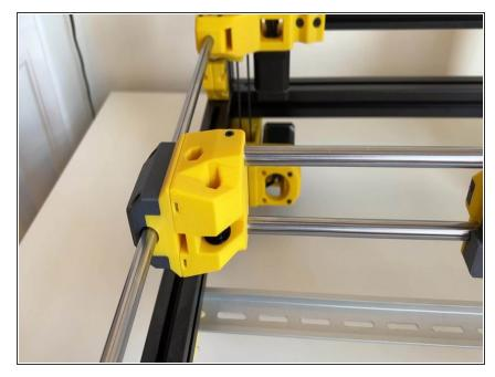
Start with 181cm B Drive Belt which is the one at the bottom. Insert the belt through the hole on the XL part.
