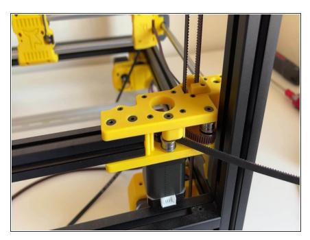
Pull the belt and continue the installation by passing through the A Drive.
