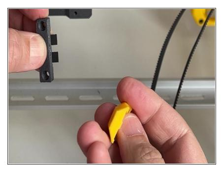
Get the other part of the belt lock and place it as seen and use an M3 x 6 screw to lock the belts.
